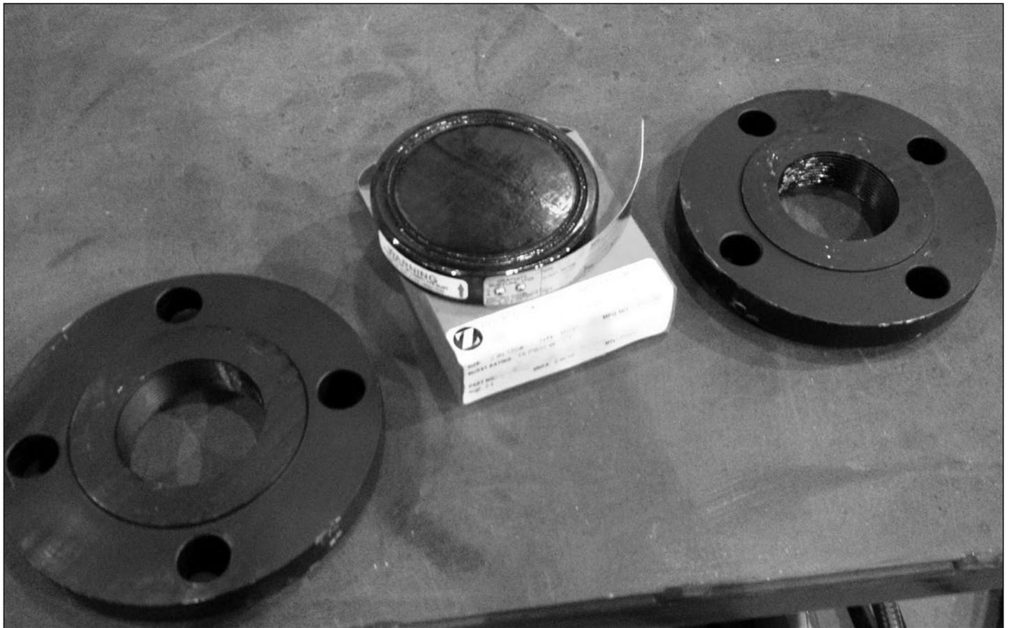
(Figure 4.1.13b) Burst disk with holders.
