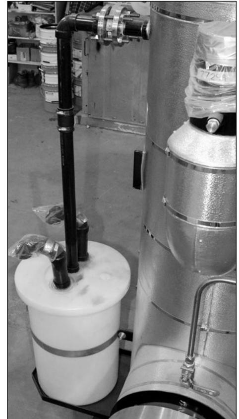
**(Note: For HPX 90 style rupture disc holder (SS)) (Note: For older style painted rupture disc holders use a torque setting of 30ft lbs on first pass and 40ft lbs on second pass)**
