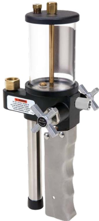
» **T-900 Series** pneumatic pressure pump features an extended range fine adjust for precise control of pressure. A built-in relief valve and dual pressure output enable safe and simple operation. The T-965 and T-975 are available with a button valve, making them capable of switching easily from pressure to vacuum generation.
