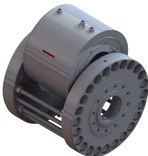
Figure 3 - The Flexflo® flanges have been jacked apart approximately 1/8" by using the inside nuts. The entire body section is then lifted out of the line. The cover plate is removed from the outlet end of the body, by removing the cap screws. The core and tube then can be pulled out of the body.
