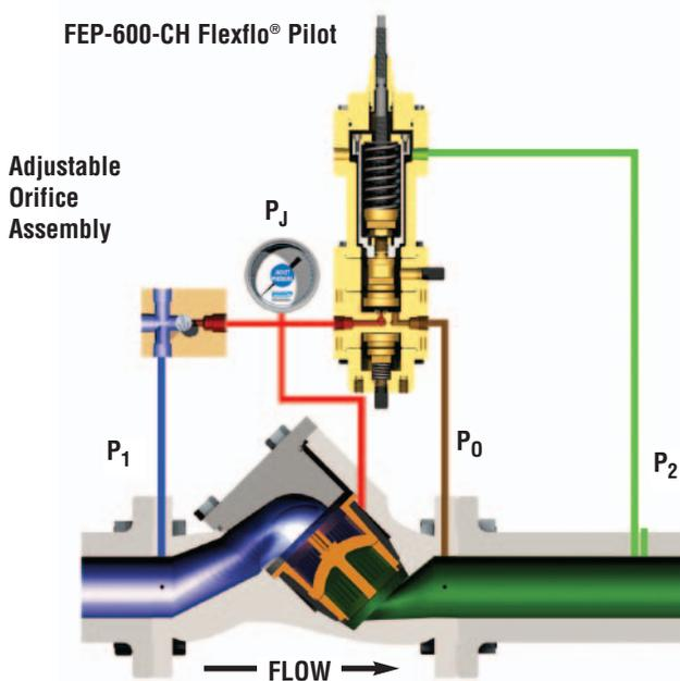
**Figure 7.2 Flexflo® Regulator Throttling**
