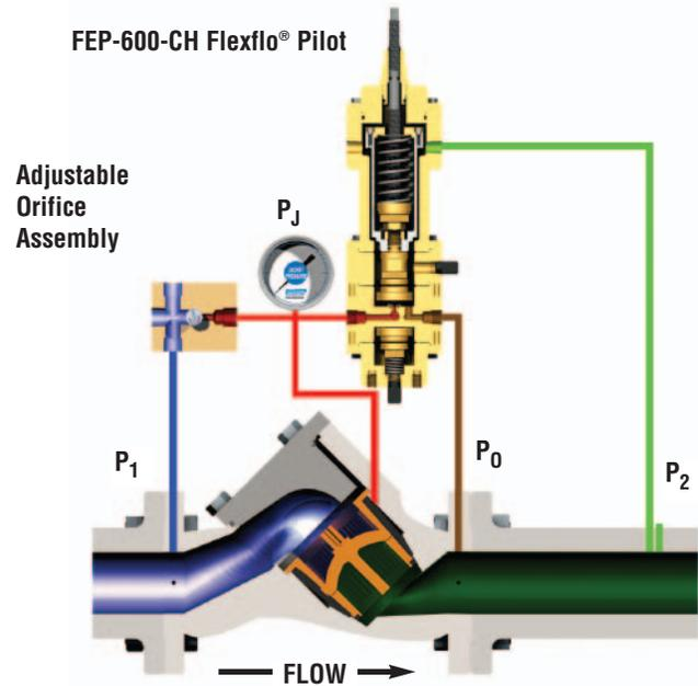
**Figure 7.3 Flexflo® Regulator Fully Open**
