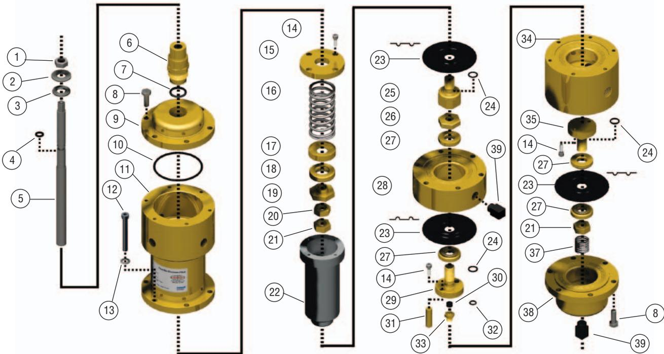
**Table 3.0 - Becker Model FEP-600-CH Flexflo® Pilot Parts Identification**
