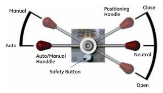
Figure 2 - MCV Handle Operating Positions
