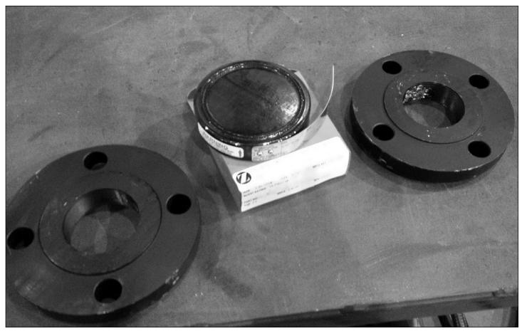
(Figure 4.1.13b) Burst disk with holders.
