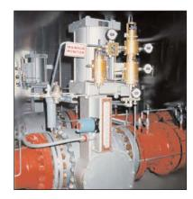
Figure 9.0 - Becker Model VRP-Pilots on Ball Valve Regs VRP-Pilot installed on RPDA Series actuator provides reliable overpressure protection in a simple instrumentation package. Note addition of the PS Non-Bleed Sensor eliminates bleed gas when control valve is full-open.
