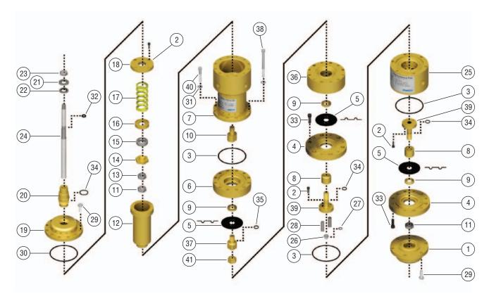
Table 3.0 - Becker Model FEP-1000-CH Flexflo® Pilot Parts Identification
