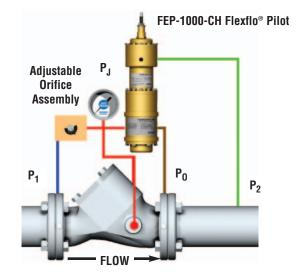
Figure 4.0 - FEP-1000-CH Flexflo® Pilot for Downstream Pressure Control
