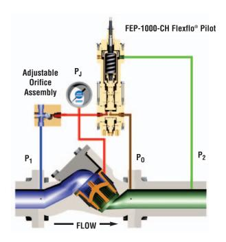
Figure 7.1 Flexflo® Regulator Fully Closed
