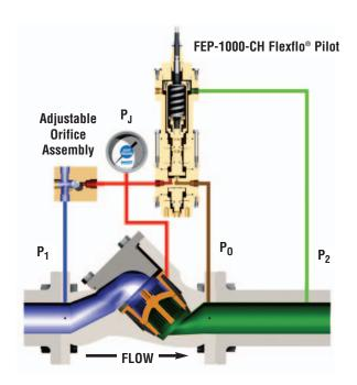
Figure 7.3 Flexflo® Regulator Fully Open
