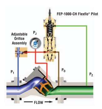
Figure 7.2 Flexflo® Regulator Throttling
