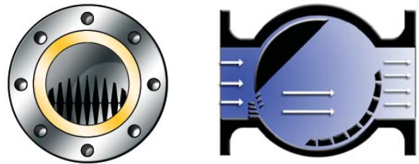
Figure 5.2 - Control valve near closed
